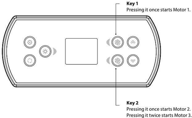
The water direction switch is on the third motor.
