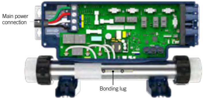
To complete the electrical connections of our in,ye control system you will need a Phillips screwdriver and a flat-head screwdriver (slotted head size between 5/16" and 3/8").
