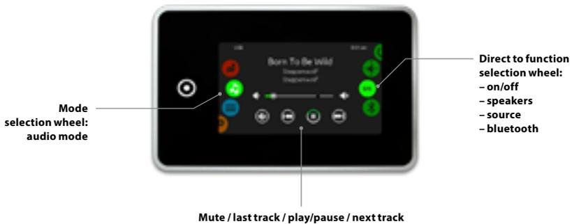
To select the audio mode, slide the left wheel up or down until the audio icon menu is highlighted in the middle.
