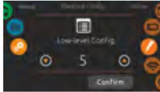
To change the low-level configuration, the number of phases and the input current of your spa system, slide the right wheel until the electrical configuration icon is highlighted in the middle.
